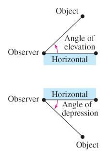
The **angle of elevation**, which represents the angle from the horizontal upward to an object.
